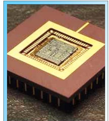
The silver square in the middle is a computer chip. The yellow color around it is gold. The whole processor of the a computer is on that chip, which is about as big as your thumb-print. It is a finely detailed
